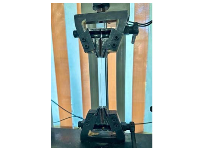
Figure 1: Fracture/deformation of retainer wire after load application.
