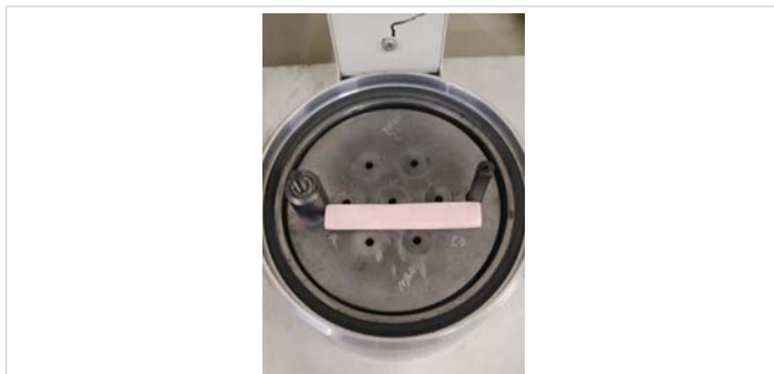
Figure 7: Sample placed in sputtering device.
