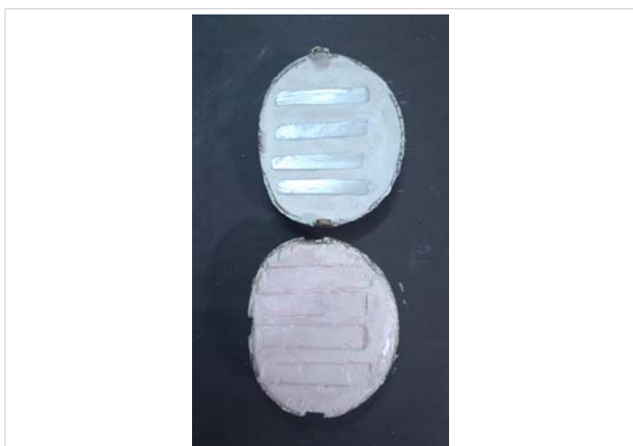
Figure 3: Mold space for acrylic specimens.
